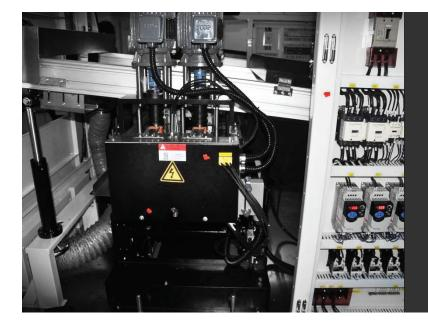
Solder pot Inlet / Outlet by motor
